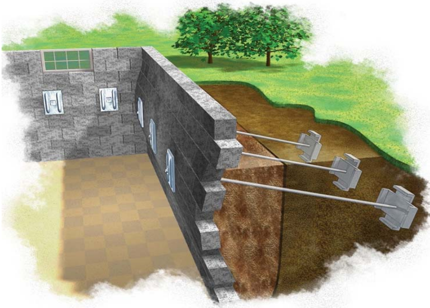
Figure 3 - Typical Wall Anchor Final
